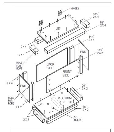
**Additional Notes.** To extend the life of the bin, caulk the lid at each joint. Attach hardware cloth to the bottom of the bin and put the bin up on bricks or risers.
